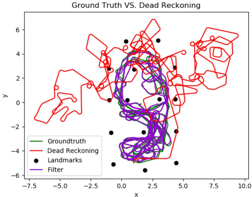
Figure 7: Particle Filter VS Ground Truth Path.
