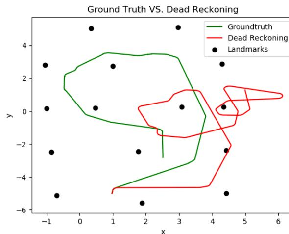
Figure 3: Dead Reckoning Pose Estimation VS Ground Truth Data, 2000 Iterations.
