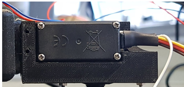
Figure 26: The added white terminal is used to measure position.
