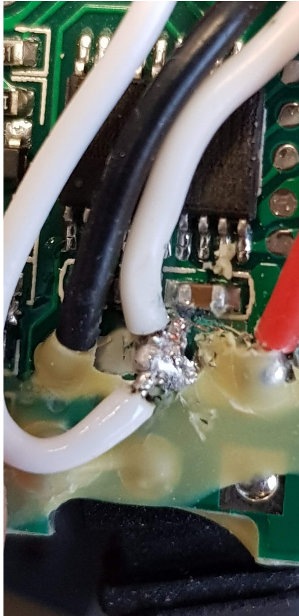
Figure 75: The additional soldered feedback terminal.
