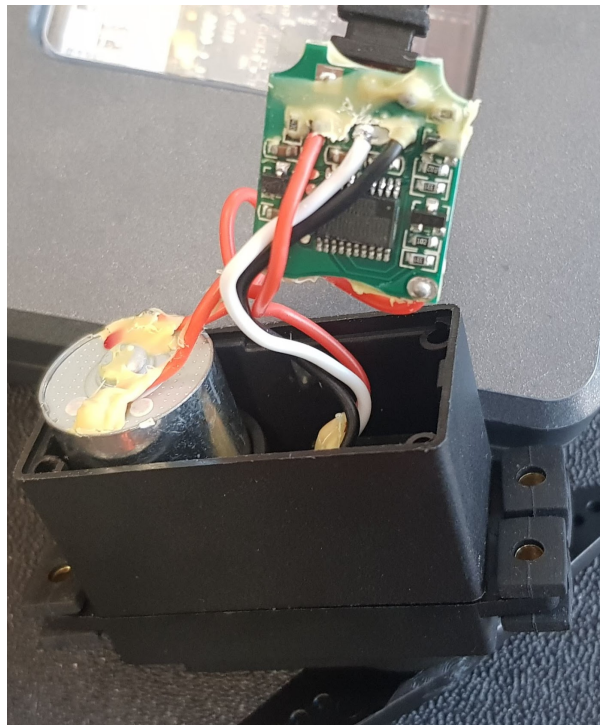
Figure 74: The motor IC with its white potentiometer terminal.
