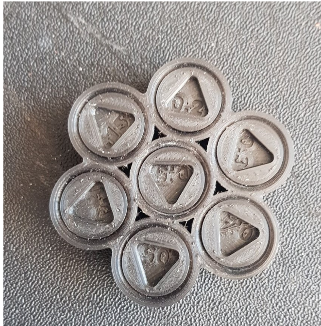
Figure 5: Calibration tool used to measure printing tolerance
